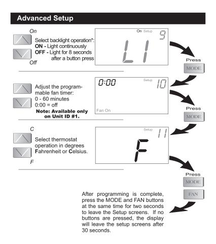
\*For increased battery life the backlight should be set to OFF unless the ACC0800 RF power supply adaptor is used to power the thermostat.
